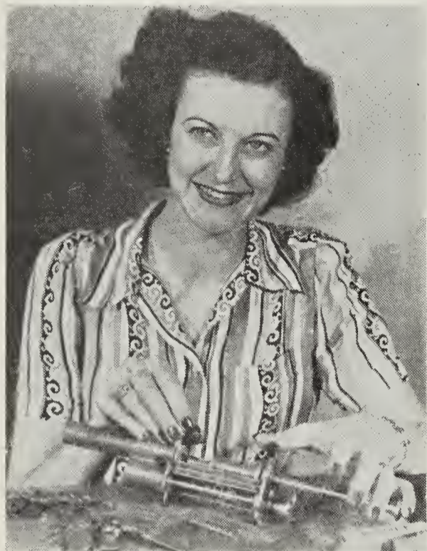
The "Rap-A-Coin" machine made by Henderize, Inc., counts and wraps pennies, nickels, and dimes. The desired tubular wrapping is put into one of three tubes, and the coins are wrapped.
